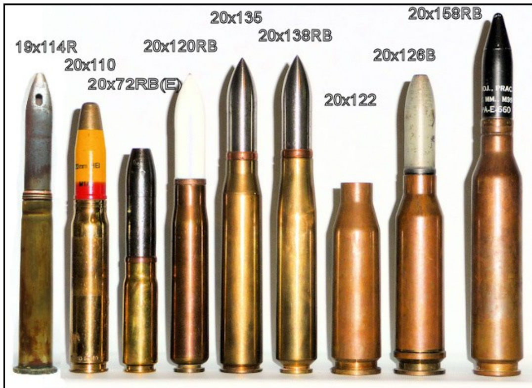
19x114R (WW1 Szakats), 20x110 (for scale), 20x72RB(E) (WW1 Ehrhard), 20x120RB Simonetta (1930s), 20x135 Polte (German pre-WW2: replica), 20x138RB (German WW2 unknown: replica), 20x122 case (post-WW2 French AA 5CG series), 20x126B (post-WW2 French AA 5CG series - used German projectiles), 20x158RB (US T5, for post-WW2 T33 aircraft gun)
